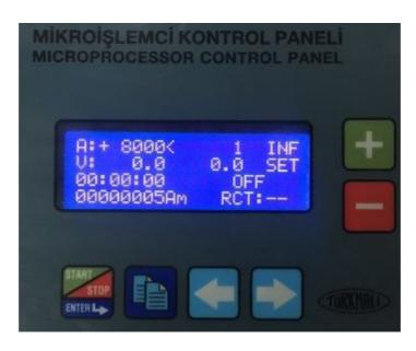
If we want to work volt controlled, we do not specify in the SET section V of the bride using the cursor and, if necessary several volt operation, (+) (-) volts to the desired key is entered.
