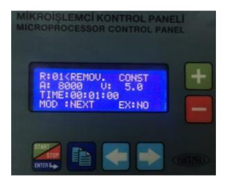
A: the rectifier of max. We are writing the stream. V: We wrote the part we want to work in several volts. Enter the time you want to work part of the time.
