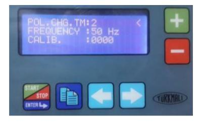
POLES CHANGE TIME: Change in the Arctic should rectifier Removal - Sets the time between the coating. Example; 2 sec after the end of disassembly, wait are made, then to start the coating process.
