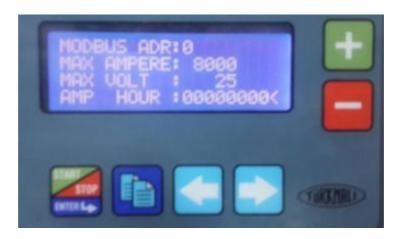
MODBUS ADR. : Modbus Address. In the automation system, the rectifier output that is what numbers refers. (+) (-) keys, rectifier sorting is done.
